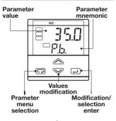
The parameter setting procedure has a timeout. If no keys are pressed for, at least, 30 seconds, the controller switches back, automatically, to the operator mode.
