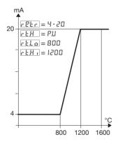
With  $r \in L$   $\alpha$  greater than  $r \in L_1$  it is possible to obtain a reverse scale.
