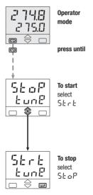
The green led MAN blinking goes on when the Fuzzy Tuning is in progress. At the end of this operation, the calculated PID terms parameter are stored and used by the control algorithm and the controller goes back to the operator mode. The green led MAN becomes off.
